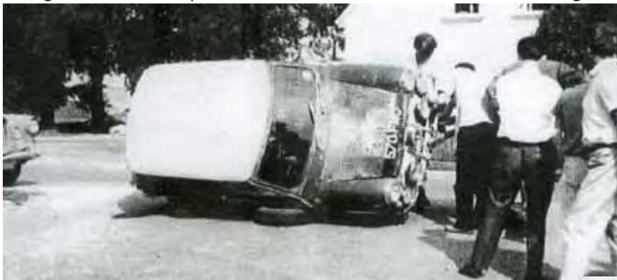
**A driveshaft joint would go no further! The Mini was tipped on its side to give the two BMC service crews better access to fit replacements**
